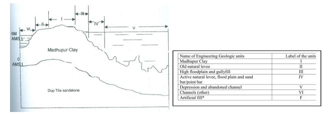
Figure 1.5 Generalised west-east cross-section showing engineering geologic units of Dhaka City (source: Shams, 1999)
