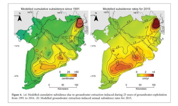
Figure 3.2 Modelled cumulative subsidence (left panel) over the last 25 years (1990-2015) and annual subsidence rates (for 2015, right panel) for the Mekong delta. The model results allow identifying subsidence hot spots, such as urban areas.
