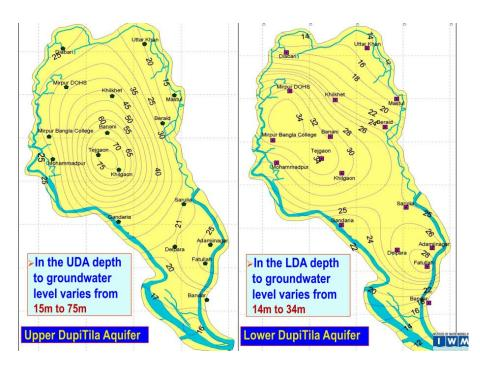
Figure 1.6 Contour map showing depth to groundwater table as on June 30 2009 in Dhaka Centre (IWM)
