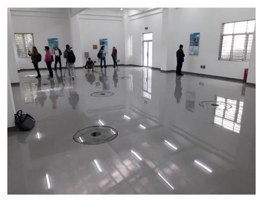
Figure 6.2 A benchmark site in Shanghai. The transparent floor tiles are the locations of the benchmarks and observation wells, each with different foundation depths and well screens (photo G. Erkens).
