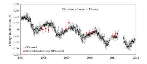
Figure 1.2 Elevation change from the Dhaka GPS record (black, with 1  $\sigma$  uncertainty in grey) (Steckler et al., 2010) and SBAS-InSAR-derived elevation change with 2  $\sigma$  uncertainty at the same location (red) (Higgins et al., 2014).
