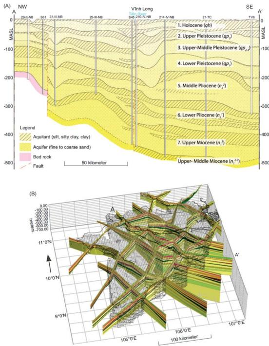
Figure 3.1 The 2.5D subsurface model based on existing data that has been constructed to serve as the geological framework for the coupled ground water subsidence model (from Minderhoud et al., 2017)
