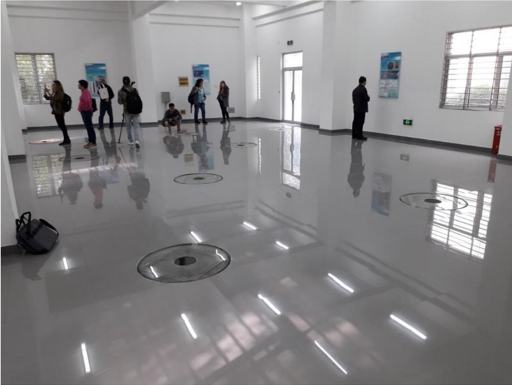
*Figure 6.2 A benchmark site in Shanghai. The transparent floor tiles are the locations of the benchmarks and observation wells, each with different foundation depths and well screens (photo G. Erkens).*
