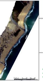
Figure 6: Constructed groynes at Keta protecting the community from erosion
