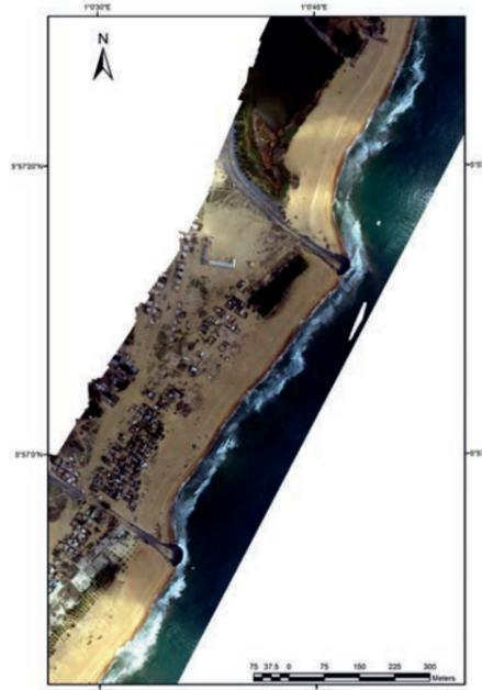
**Figure 6:** Constructed groynes at Keta protecting the community from erosion
